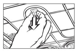
■ Pull and turn the fastener on the grill element to release it.
